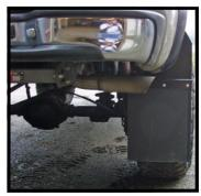
Support Bracket Installation required for rear mud flaps. This bracket is not required for shorter Mud flaps under 16" in length due to their lighter weight.
